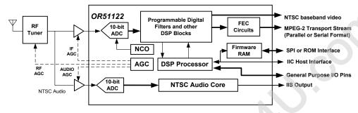
The OR51122 builds on Oren's powerful and efficient demodulator DSP technology and adaptable filter blocks controlled by a central DSP processor, adding accelerated 8-VSB for ATSC demodulation. The OR51122 also processes NTSC video signal and translates the incoming signal to baseband output. BTSC audio is demodulated and decoded. This proprietary implementation results in many application benefits:
